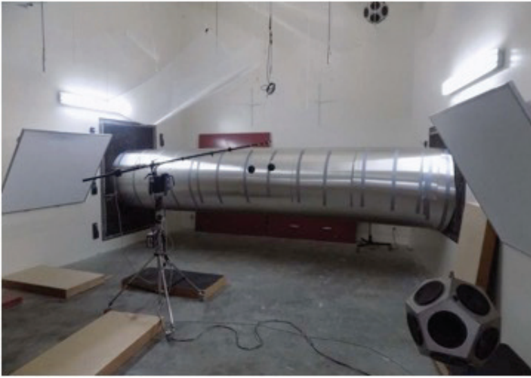
Figure 2. A sound room is used to measure insertion loss after acoustic insulation is applied, per ISO 15665.
