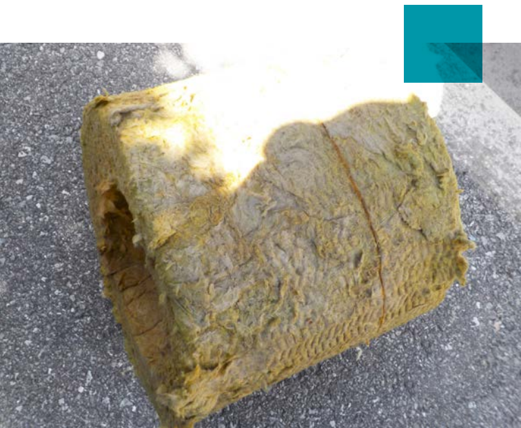
ROCKWOOL WR-Tech insulation after three years at 120°C to 140°C.
