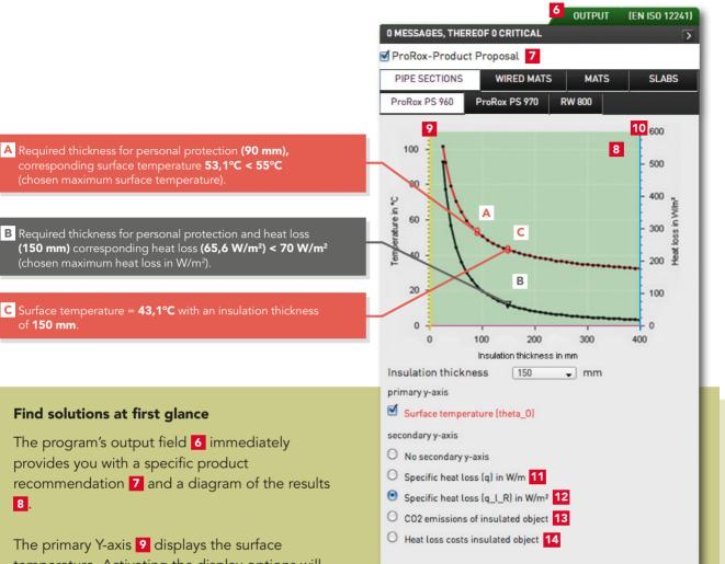
corresponding surface temperature 53,1°C < 55°C (chosen maximum surface temperature)
