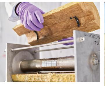
A technician prepares an ASTM G189 test cell by applying a section of ProRox<sup>®</sup> PS 965 with CR-Tech™ around a pipe section containing carbon steel coupons. ASTM G189 is the standard guide for laboratory simulation of CUI. This test can be used to simulate an accelerated corrosion environment to compare corrosion rates of different combinations of insulation systems.
